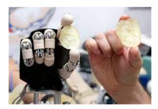
The bionic hand looks like the real one, although it is made by metallic materials and its color is metallic too. It has fully articulated joints in the area of the knuckles, an individual motor for each digit and sensors in socket pick up myoelectric signals from arm muscles to make full range of movements.
